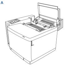
**WARNING!** The printer must be kept level at all times unless ALL oil is removed.
